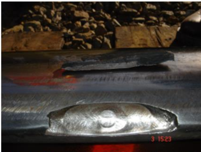
Figure 1a. DSS defect originating 6 mm below the gauge corner was detected by the ultrasonic car.
